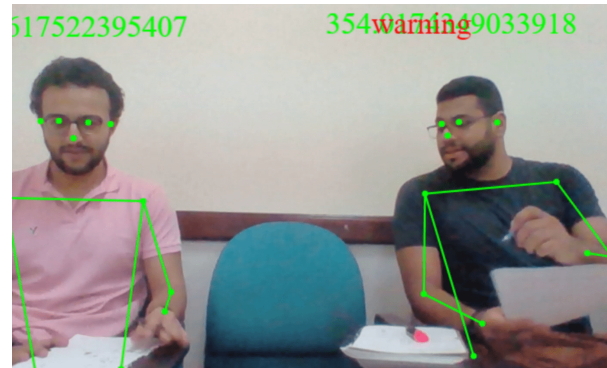
Fig. 5. Demonstrates the detection of an abnormal head angle that results in a warning.
